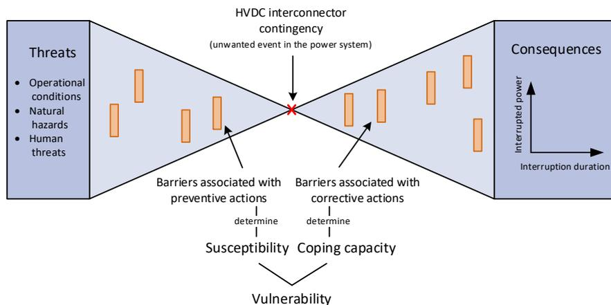
**Figure 1. Bow-tie model for vulnerability analysis of HVDC interconnector contingencies, based on [6].**
