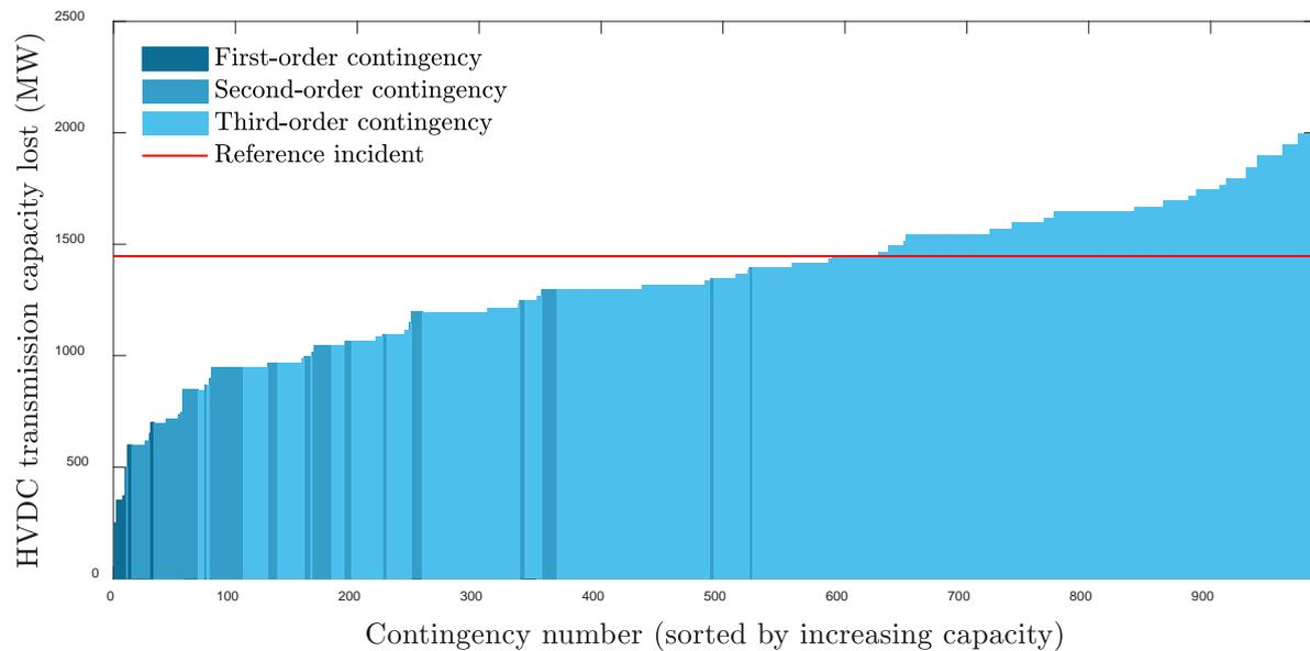
**Figure 3. The severity of HVDC interconnector contingencies in terms of the maximum amount of transmission capacity lost, for the HVDC interconnectors that are currently (2018) operational and connected between the Nordic synchronous area and another synchronous area.**
