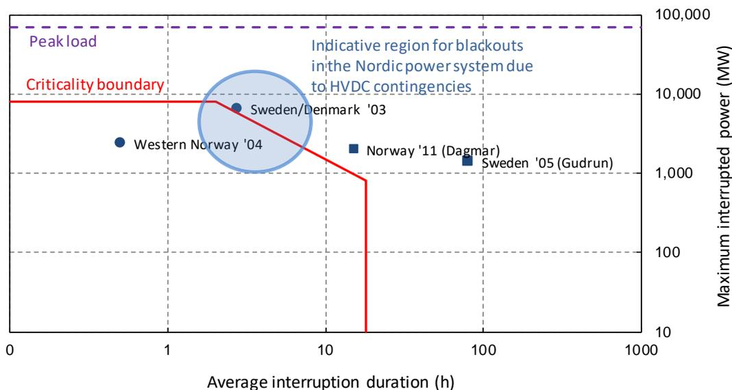
**Figure 2. Consequence diagram indicating possible consequences for blackouts in the Nordic synchronous area due to HVDC contingencies, compared with historic blackout events, based on [6], with the criticality boundary suggested in [9] and peak load in the system as given in [11].**
