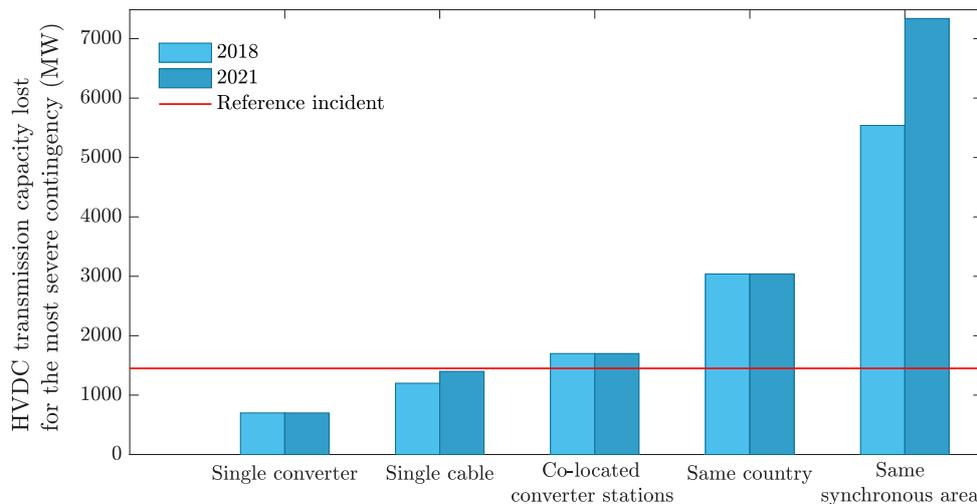
**Figure 4. The severity of the most severe HVDC interconnector contingencies for different levels of co-location of the HVDC converters.**
