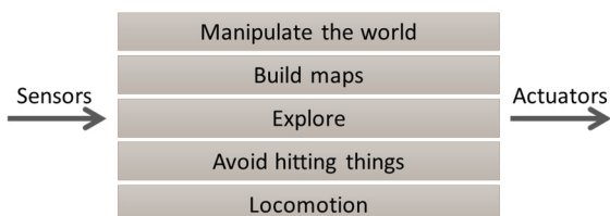
Figure 6. Layered control system according to Brooks [19]
