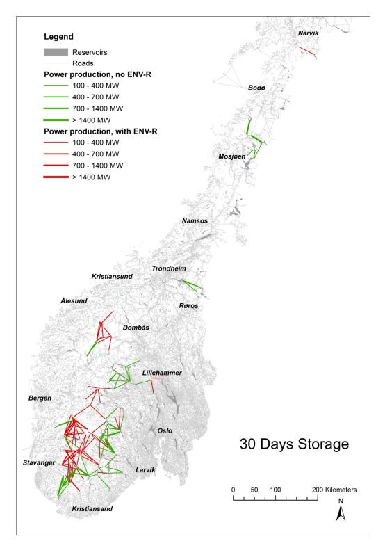
Figure 12: PSH potential for 30 days storage duration and minimum power production of 100 MW, calculated using the T-Mode. Green lines indicate no conflicts with environmental restrictions. Red lines stand for PSH connections where these restrictions are violated.
