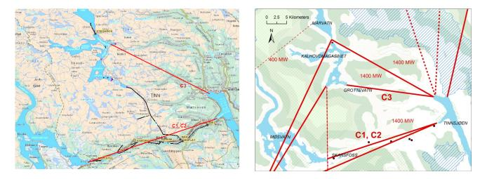
Figure 6: The Møsvatn-Tinnsjø-Kallhovd/Mår area with the PSH cases suggested by Solvang et al. (2012, left) and the GIS-screening results obtained using the P-Mode for 400, 700 and 1400 MW. Dashed lines: PSH lines which are in conflict with the environmental restriction zones.
