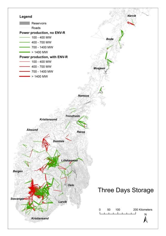
Figure 10: PSH potential for three days storage duration and minimum power production of 100 MW, calculated using the T-Mode. Green lines indicate no conflicts with environmental restrictions. Red lines stand for PSH connections where these restrictions are violated.
