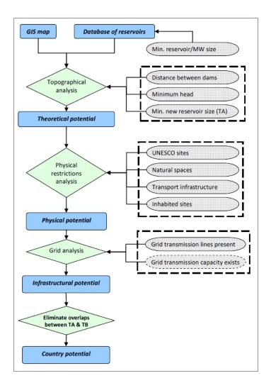
Figure 1: Methodology flow chart for the PSH potential study performed by Arántegui et al. (2011)
