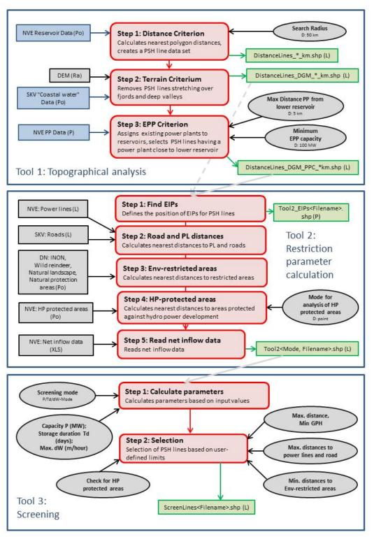
Figure 4: Flow chart of the Tool. Grey: user-defined parameters (ellipse) or input data sets (rectangle). Blue: Fast implemented input data sets. Green: Output data sets. Ra = Raster data. Vector data: Po = Polygon, P = point, L = Line.
