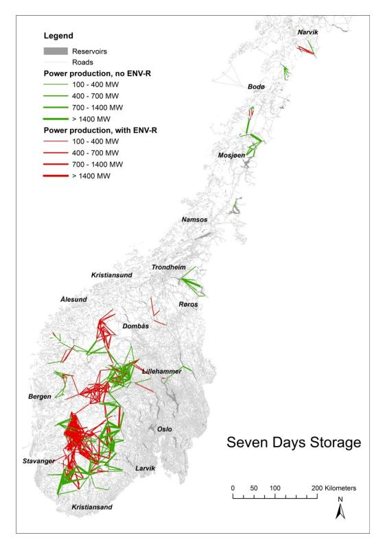
Figure 11: PSH potential for seven days storage duration and minimum power production of 100 MW, calculated using the T-Mode. Green lines indicate no conflicts with environmental restrictions. Red lines stand for PSH connections where these restrictions are violated.
