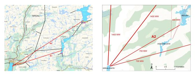
Figure 5: The Tonstad Case from Solvang et al. (2012, left) and results of the GIS-screening for 400, 700 and 1400 MW (P-Mode). Dashed lines: PSH lines which are in conflict with the environmental restriction zones.
