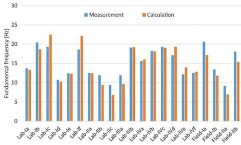
Fig. 2 Comparison of calculated and measured fundamental frequency.
