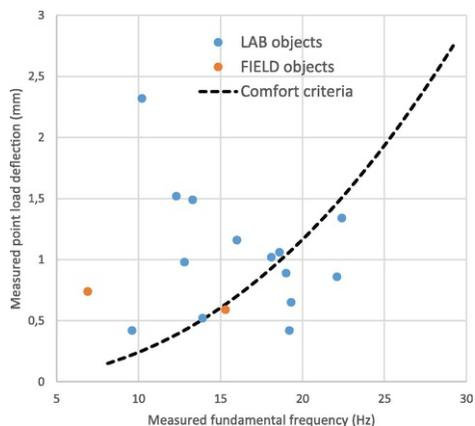
Fig. 9 Evaluation of floor vibration properties from measurement results.
