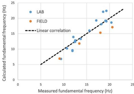
Fig. 3 Comparative analysis of calculated and measured fundamental frequency.
