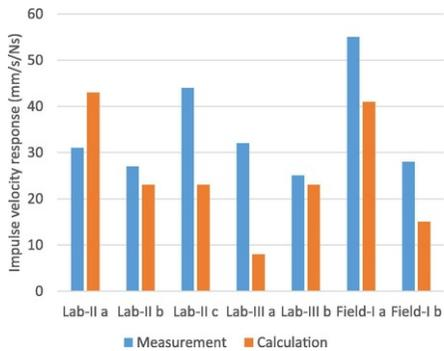
Fig. 4 Comparison of calculated and measured maximum impulse velocity responses.
