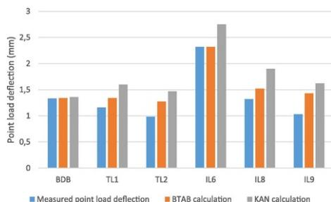
Fig. 1 Measured and calculated deflection from 1 kN point load at midspan.
