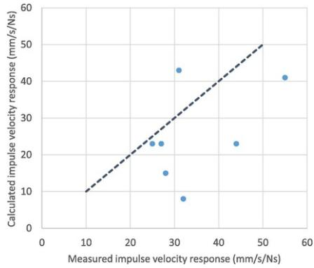
**Fig. 5** Comparative analysis of calculated and measured maximum impulse velocity responses.
