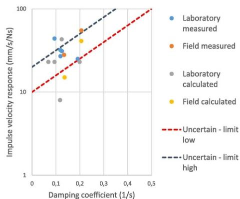
**Fig. 8** Evaluation of floor vibration properties according to [2].
