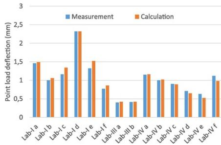
**Fig. 6** Comparison of calculated and measured point load deflection.
