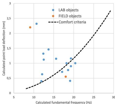
Fig. 10 Evaluation of floor vibration properties from calculated results.
