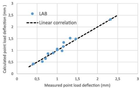
**Fig. 7** Comparative analysis of calculated and measured point load deflection.
