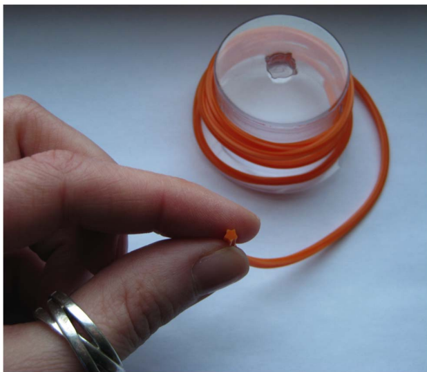
Figure 3. Silicone string for mimicking portal veins. doi:10.1371/journal.pone.0064180.g003
