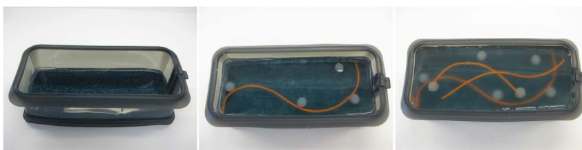
Figure 4. Manufacturing multimodal phantom. Left: step 19 of the protocol; Middle: step 22 of the protocol; Right: the end result of the protocol – multimodal phantom mimicking liver tissue.
