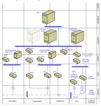
Fig. 2. SGAM component layer for the combination of controls required for the WoC concept. Source [12].
