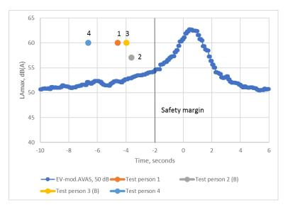
Figure 11. Example of analysis and results of one run (Test 5). Persons 2 and 3 are visually impaired
