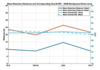
Figure 3. Mean detection distance and overall SPL, with background noise level of  $60 \text{ dB}^{17}$
