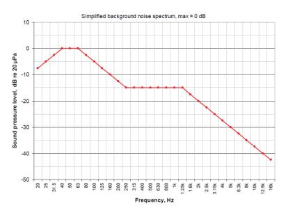
Figure 7. Normalized noise spectrum used as a background noise signal<sup>10</sup>
