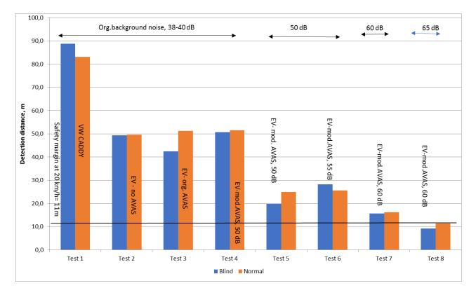
*Figure 13. Comparison of detection distance between the group of blind/visually impaired and group of normal seeing*
