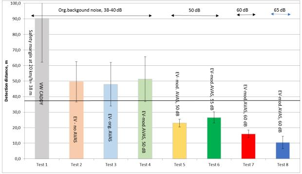
Figure 14. Detection distance with a safety margin of 38 m
