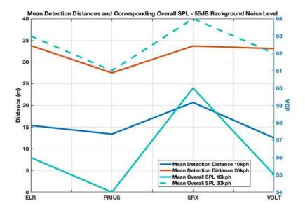
Figure 2. Mean detection distance and overall SPL, with background noise level of 55 dB<sup>17</sup>
