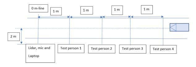
Figure 4. Layout of test area
