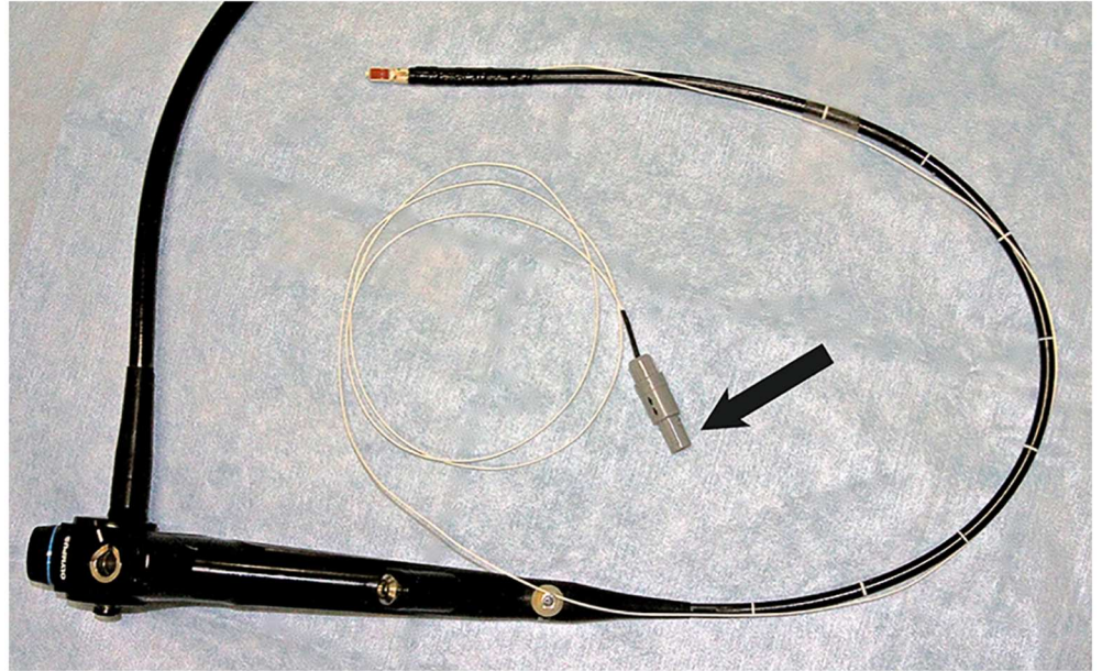
Fig 2. Experimental EBUS bronchoscope. The sensor for electromagnetic tracking was attached close to the convex probe in the tip of the bronchoscope. The connector to the sensor (arrow) was plugged into the control unit of the electromagnetic tracking system.
