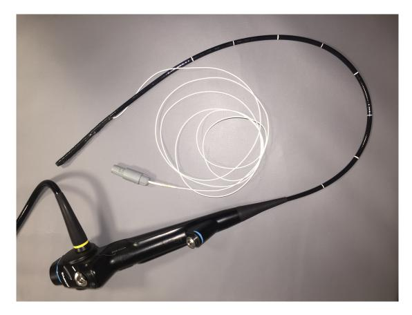
Figure 4: The bronchoscope with a position tracking sensor mounted close to the tip.
