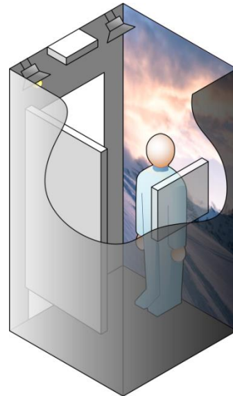
Fig. 3. The customer sees itself as standing in a landscape when trying on clothes for skiing. Product information can be provided through the magic mirror.
