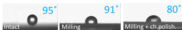
Figure 5: Contact angle measurements (3 \mu\text{L} drop volume) of COP surfaces before milling ("intact"), after milling, and after milling and chemical polishing.
