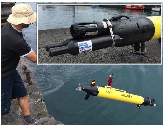
(a) Launching the LAUV-Xplore-1 off of a pier in the island of Horta for testing. Inset image shows the nose cone of the AUV with an experimental miniature holographic camera.
