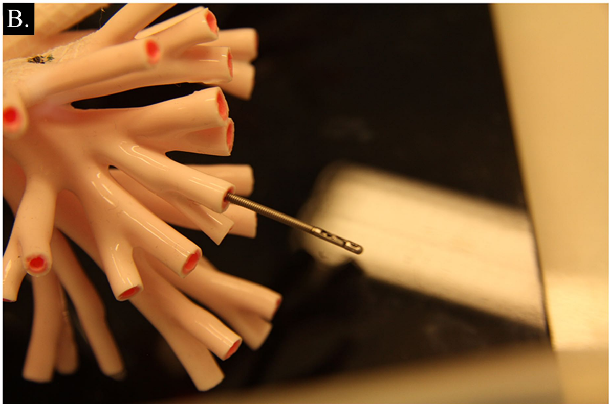
Figure 4. A): The experiment setup B): Forceps reaching the target and exiting the phantom airway at the correct branch.
