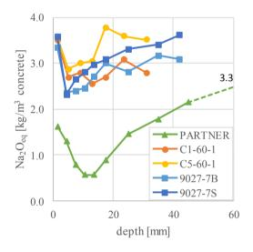
Fig. 7 : The  $Na_2O_{eq}$ -profiles (in kg/m<sup>3</sup>) concrete in function of the depth of the exposed surface (in mm) obtained by CWE for the examined samples. The 3.3 kg/m<sup>3</sup>  $Na_2O_{eq}$  indicated in the graph reflects the content determined in a section taken at a depth of approx. 100 mm-150.
