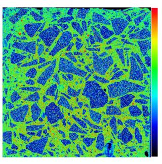
**Fig. 10 :** K-map of a sawn concrete surface of the C5-60-1 sample. The closer the color is to red the higher is the relative content of K. The dimensions of the sample are 70x70 mm.
