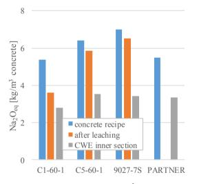
**Fig. 15 :** The  $Na_2O_{eq}$  content (in kg/m<sup>3</sup> of concrete) based on the concrete recipe (Table 2), the average alkali content in the sample after leaching, and the alkali content in the inner section of the concrete sample obtained by CWE.
