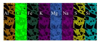
Fig. 5 : Elemental maps determined with the  $\mu$ XRF of section 30-40 mm of sample C5-60-1.
