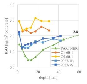
**Fig. 8 :** The K<sub>2</sub>O-profiles (in kg/m<sup>3</sup>) concrete in function of the depth of the exposed surface (in mm) obtained by CWE for the examined samples. The 2.8 kg/m<sup>3</sup> K<sub>2</sub>O indicated in the graph reflects the content determined on a section taken at a depth of approx. 100 mm-150.
