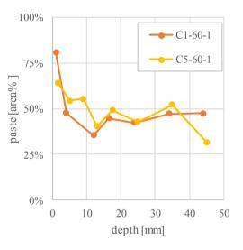
**Fig. 14 :** The area% of paste in the sections as a function of the depth from the surfaces determined using the phase differentiation with the  $\mu$ XRF.
