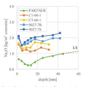
Fig. 9 : The Na<sub>2</sub>O-profiles (in kg/m<sup>3</sup> concrete) in function of the depth of the exposed surface (in mm) obtained by CWE for the examined samples. The  $1.5 \text{ kg/m}^3 \text{ Na}_2\text{O}$  indicated in the graph reflects the content determined on a section taken at a depth of approx. 100 mm-150.
