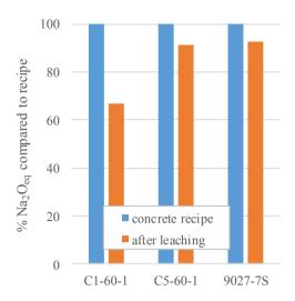
**Fig. 16 :** The % Na<sub>2</sub>O<sub>eq</sub> left in the concrete after leaching compared to the alkali content initially in the concrete (concrete recipe, Table 2).
