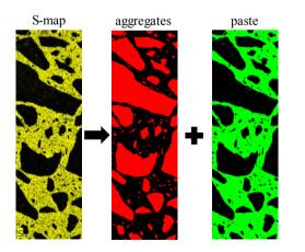
**Fig. 6**: Demonstration of the differentiation between aggregates (red) and paste (green) in section 30-40 mm of sample C5-60-1 using the S elemental map.
