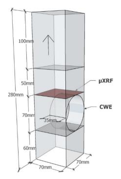
Fig. 3 : Sampling from prism C1-60-1 and C5-60-1.
