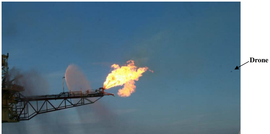
Figure 4.5 Close up view of flare with smoke plume and drone in background.
