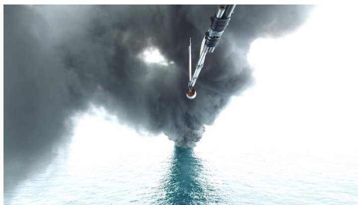
Figure 5.2 View from the drone of how a rising smoke plume from an In-Situ Burn of Oil divides into two counter-rotating vortices. This image was taken during NOFO's 2018 Oil on Water exercise. The plots of data in Figures 5.3 through 5.5 depict the presence of the two counter-rotating vortices that were encountered during Flight 14.
