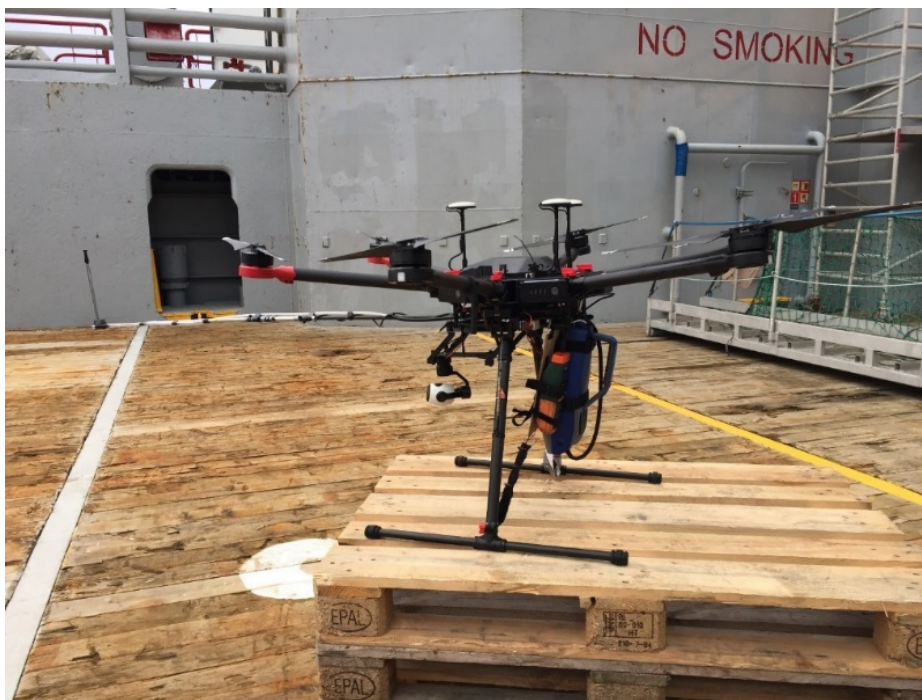
Figure 4.1 View of the hexacopter drone instrumented with an anemometer and a DustTrak aerosol monitor. Instrument sensors or intake to the instrument sensors that were utilized for collecting smoke plume data were placed on a support arm upwind of the drone's propeller downwash.
