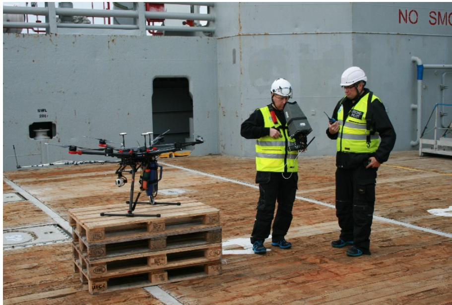
Figure 4.2 View of the hexacopter drone instrumented and both Maritime Robotics drone pilots. A hood-screen was used to pilot the drone. The stack of pallets reduced magnetic interference to the drone's compass.
