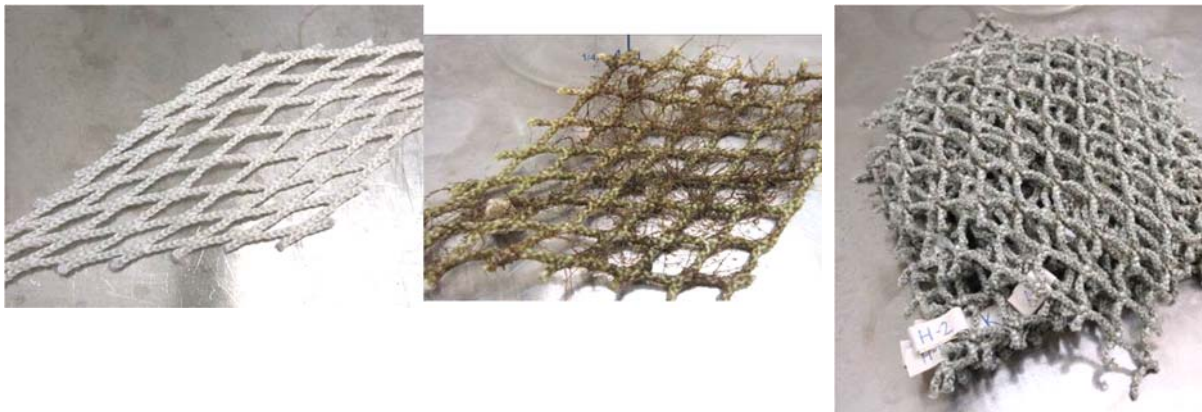
Figure A-1: Netting materials subjected to chemical exposure tests. From left: N1, N1_bf and N2.
