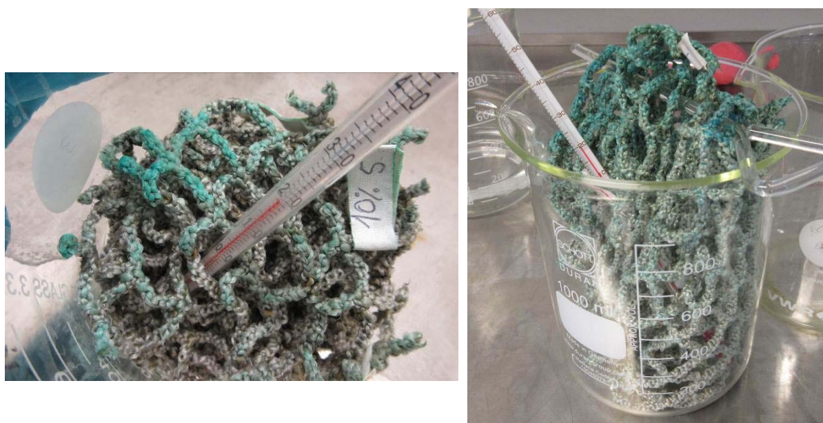
Figure A-4: Used netting with copper residuals, N 2 , subjected to 10 % Aqua Des (left) and concentrated Aqua Des (right).
