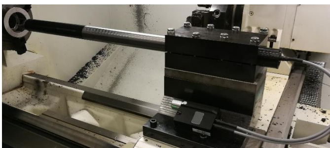
Fig. 1. The tool with electronics for wireless sensor data transfer to user.
