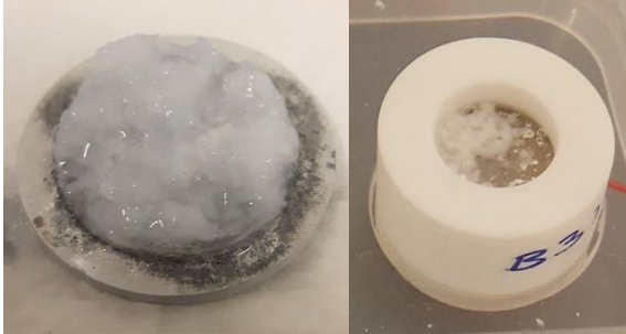
Fig. 10: Deposits on aluminum specimen at TCD of 80 A/mm 2 at 50 Hz (left) and TCD of 40 A/mm 2 at 200 Hz (right).
