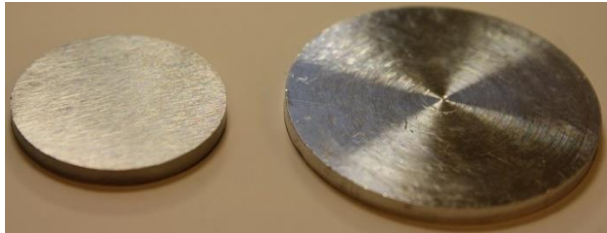
Fig. 2: Polished specimens of steel (left) and aluminum (right)
