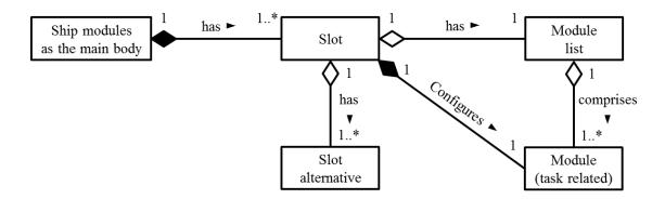
Figure 3. Description of ship modules, slots, and task-related modules using a class diagram in the unified modeling language.
