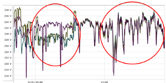
Figure 7 RMS voltage metered (Cycle by cycle), before and after the inverter connected to the battery was used for voltage support
