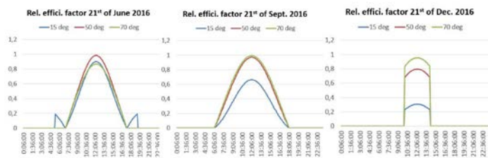
Figure 3 Relative efficiency factor of a PV panel at different days, using 15°, 50° and 70° elevation, panel pointing at south
