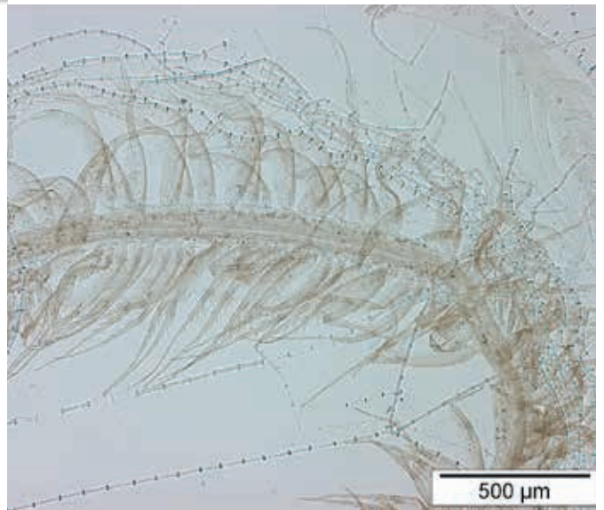
Treated (2.5 M NaOH, 50°C, 40 minutes) chicken feathers seen by microscope.
