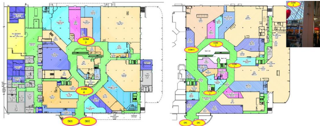
Figure 92. Ground and First Floor monitoring sensors position in CitySyd
