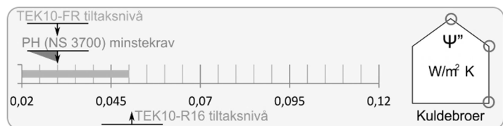
Figure 14 Typical level of the combined thermal bridge factor normalised per m 2 of heated floor area.
