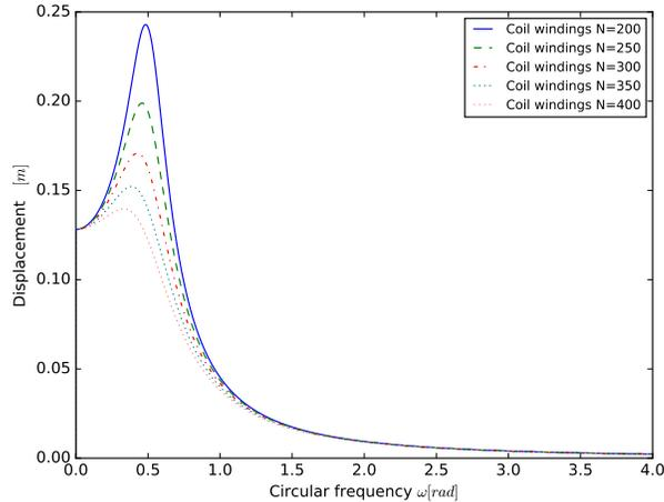
Figure 3: Maximum displacement range of the hydraulic piston.
