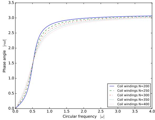
Figure 4: Phase angle between piston displacement and wave amplitude.
