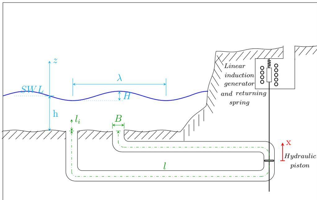
Figure 1: Schematic of the harmonic pressure wave energy converter.
