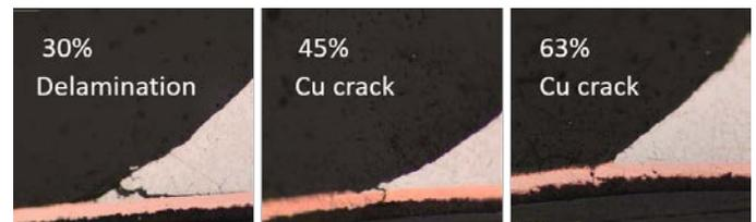
Fig. 9. Cross section of failed BiSn interconnects. With  $T = 30\%$  of  $T_{fail}$ , the main failure mode was delamination of the BiSn from the Cu tracks. For  $T = 45\%$  and 63% of  $T_{fail}$ , the main failure mode was a crack in the Cu tracks.
