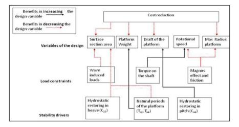
Figure 1: Constraints in developing baseline design [3]
