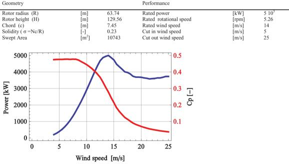
Figure 3: 5 MW DeepWind baseline design power curve(blue) and C<sub>P</sub> (red)
