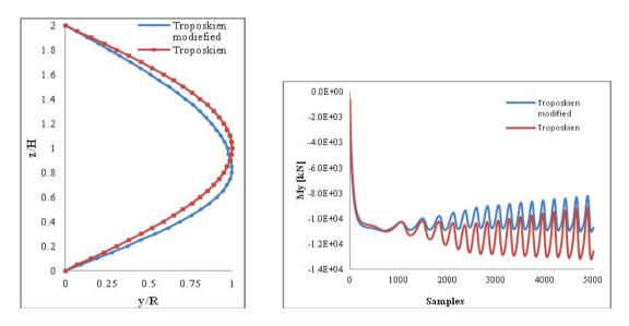
Figure 4: Left: Two different blade shapes according to two different operational conditions. Right: Loads corresponding to the two different rotor shapes [3].
