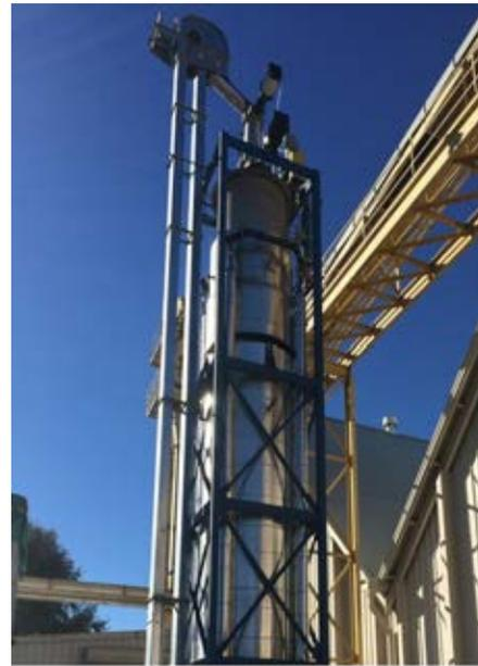
Figure 2: A 2MWth circle-draft biomass gasifier
