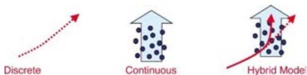
Figure 2: Single Lagrangian parcel trajectory (left side), the continuous droplets travels with local average velocity (middle), hybrid model in which consider the impact of the other existing droplets on the Lagrangian trajectory (right side)
