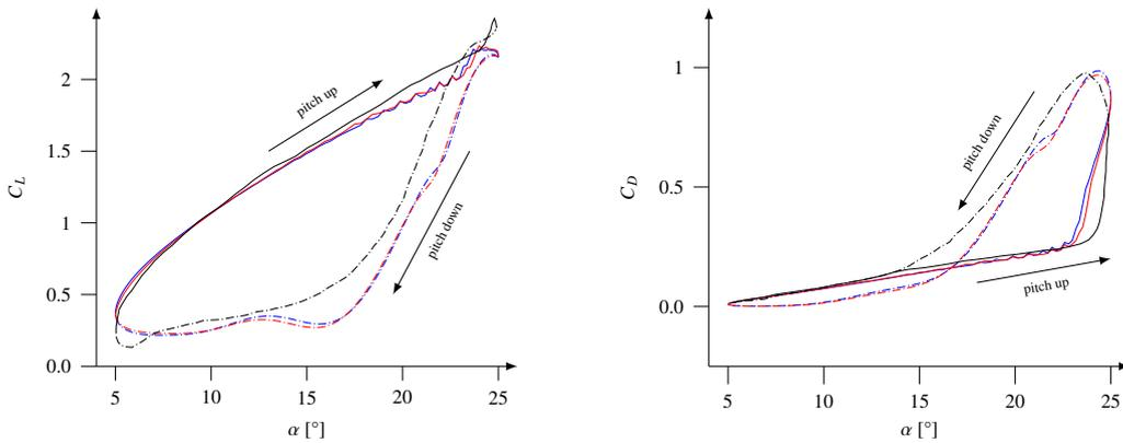
Fig. 5: Aerodynamic coefficients during a periodic cycle, with – experiments from [19], –  $p = 1$  and –  $p = 2$ .
