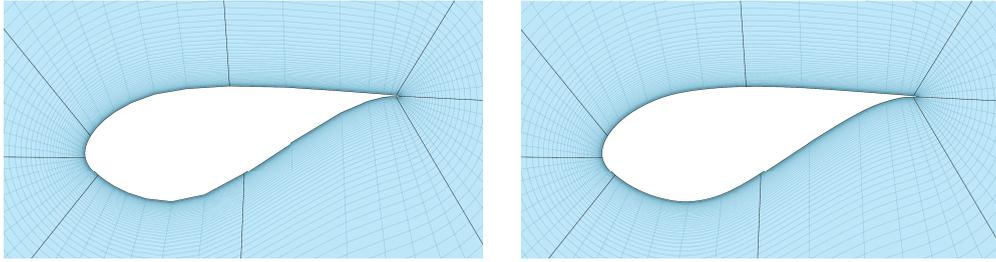
Fig. 1: Representation of a cross section of a blade using linear elements (left) and cubic splines (right).
