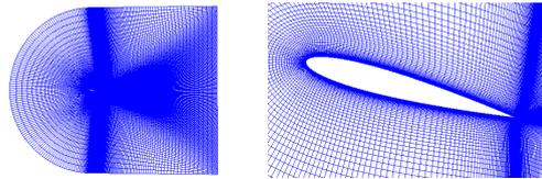
Fig. 3: C-mesh of the flow domain.
