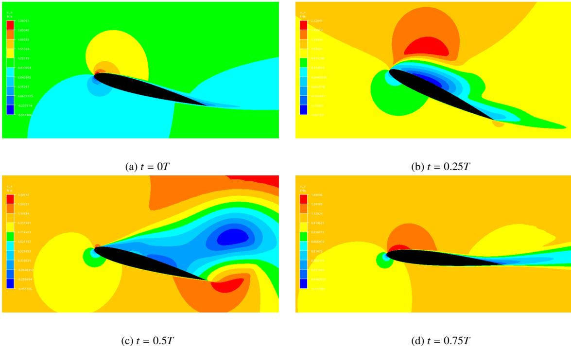
Fig. 4: Snapshots of the horizontal velocity during different phases of the periodic cycle.
