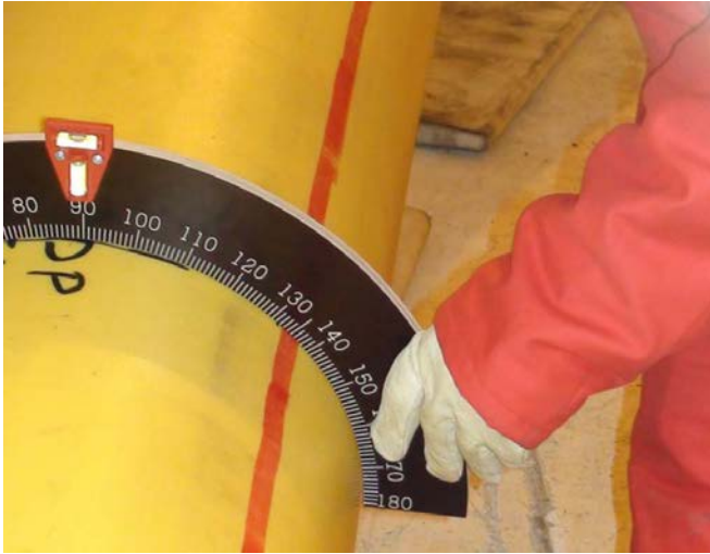
Figure 4 Roll angle measurement
