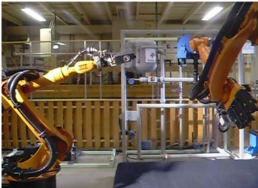
Fig. 9. KUKA KR16 industrial robot used in the experiments.
