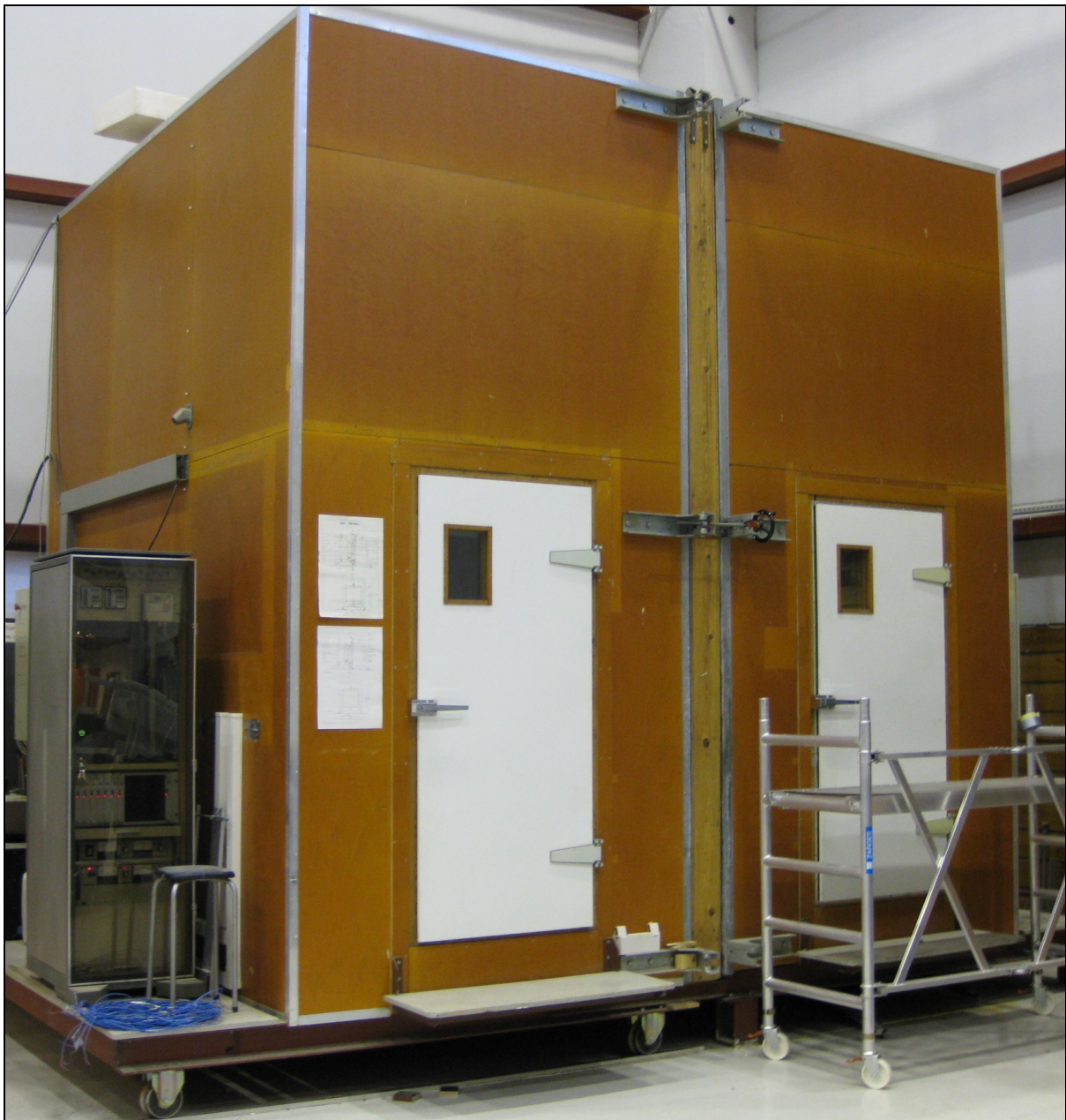
Figure 2 Photograph of the guarded hot box. The hot box is to the left and the cold box is to the right, with the sample in between.
