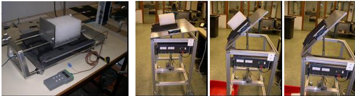
Figure 9. Friction coefficient determination between snow and roofing by method A – horizontal plane applied pulling force method (first photo to left) and method B – inclined plane slip method (three photos to right). (Photo: SINTEF Building and Infrastructure).
