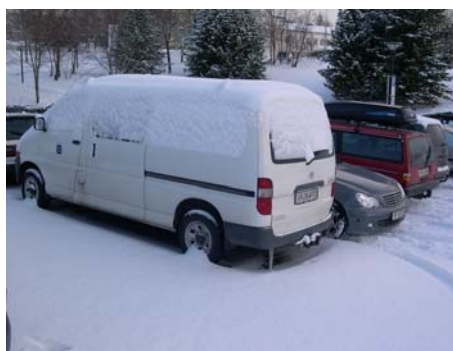
Figure 12. Snow covering almost vertical car windows. (Photo: SINTEF Building and Infrastructure).
