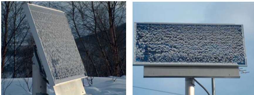
Figure 11. Snow covering a solar cell panel at an inclination angle of 70°. Day 1, blue sky, -19°C and clean panel → Day 2, light clouding, fresh snow, -13°C ⇒ Panel covered with snow. (Photo: NTNU).
