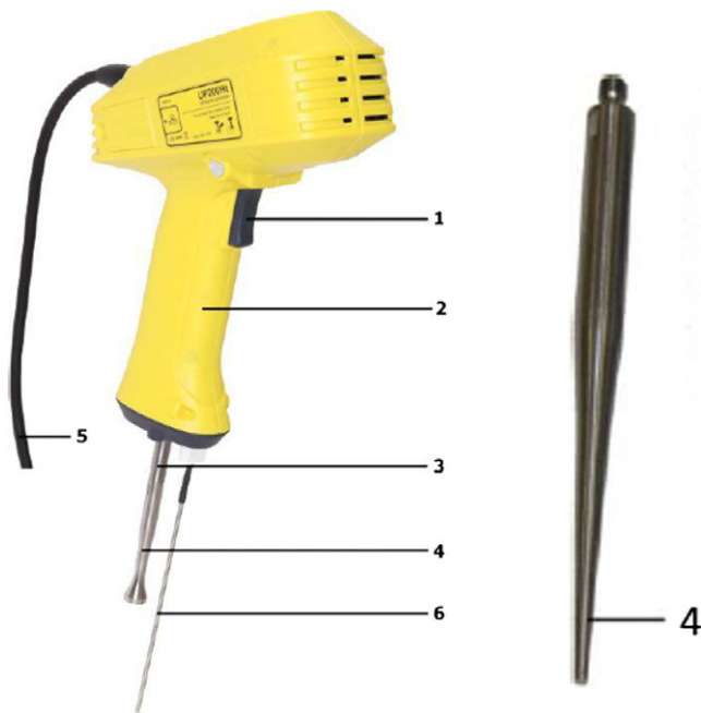
FIGURE 1 Left: Ultrasonic Processor UP200Ht from Hielscher. 1-activation trigger, 2-handhold, 3-sonotrode attachment, 4-sonotrode, 5-power cord, 6-temperature probe. Right: The Sonotrode used in the experiments (S26d2, 2 mm). Photos: Hielscher, Germany, ©www.hielscher.com, 2016
