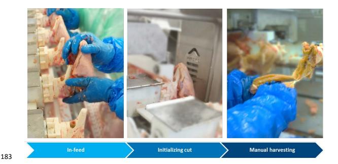
Figure 1. Stages in the manual harvesting of front half chicken fillets, preceded by manual in-feed, mechanical incision for the
