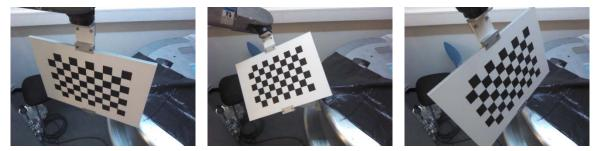
284 Figure 6. Examples of images of the calibration board used for eye-to-hand calibration of the Kinect v2
