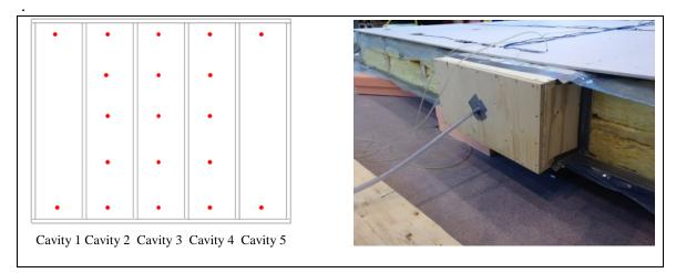
**Figure 5.** Equipment used for measuring equivalent air permeability of the insulated cavities of the test section. Red dots indicate positions of air pressure measurements. Test section seen from the cold side. I
