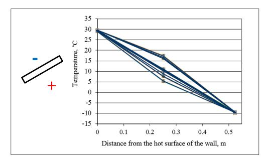
**Figure 10.** Temperature on the cold and warm surfaces of the test section and in the centre of the glass wool insulation at a 30-degree inclination (pitched roof).
