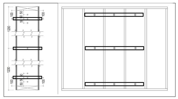
**Figure 2.** Positions of the 39 thermocouples, indicated by dots, inside (crossection to the left) and on the cold and warm surfaces of the test section (elevation view to the right). Frames indicate the position of the thermocouples included in Figure 9-12.
