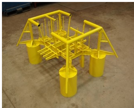
FIGURE 1. EXAMPLE OF SUBSEA STRUCTURE WITH SUCTION ANCHORS. MODEL OF THE GJØA TEMPLATE.
