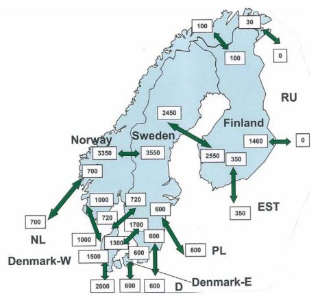
Figure 7 Expected cross border available trading capacities in 2012 (MW) [7]
