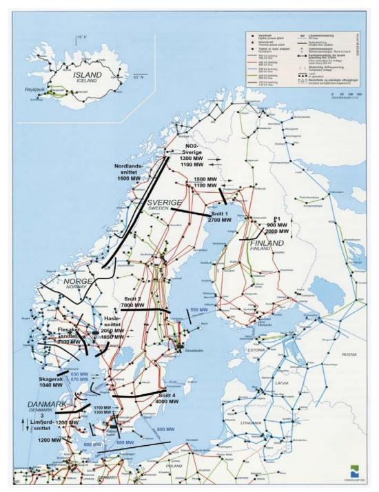
Figure 6 The transmission system in the Nordic region with relevant transmission constraints [5].
