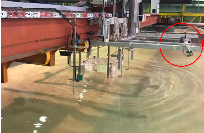
Figure 9: Aluminum frame attached to carriage on which optical motion tracking cameras (in red circle) were also mounted.
