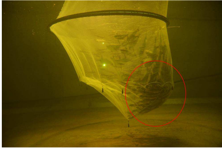
Figure 12: Side view photo from the live fish experiment with U = 0.10 \text{ m/s} . The area encircled indicates the observed touching area between the fish and the net
