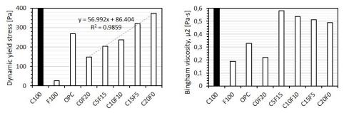
Fig 1 - Dynamic viscosity of cement blends Fig 2 - Bingham viscosity of cement blends (w/b = 0.36) (w/b = 0.36)
