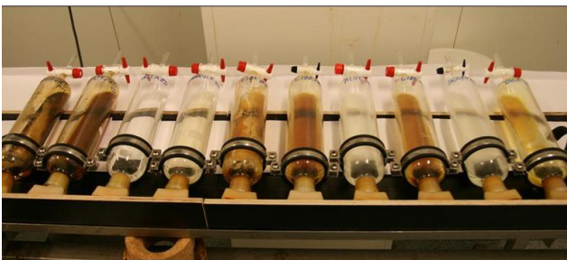
Figure 6-2 Examples from the tilting cylinder method /rocking table test of different oils/residues from the TOF project
