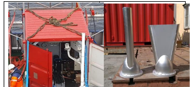
Figure 7-4 Left: A complete container based bow boom system for mechanical dispersion by high capacity water flushing and use of dispersants. Right: Deflector nozzles
