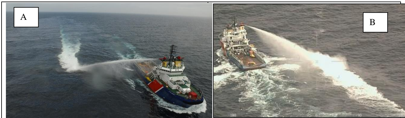
Figure 8-6 Water flushing using SB Fi-Fi monitor on MS Strilborg. Drone video by Maritime Robotics (A) and ©Finnish Border Guard / SYKE (B)
