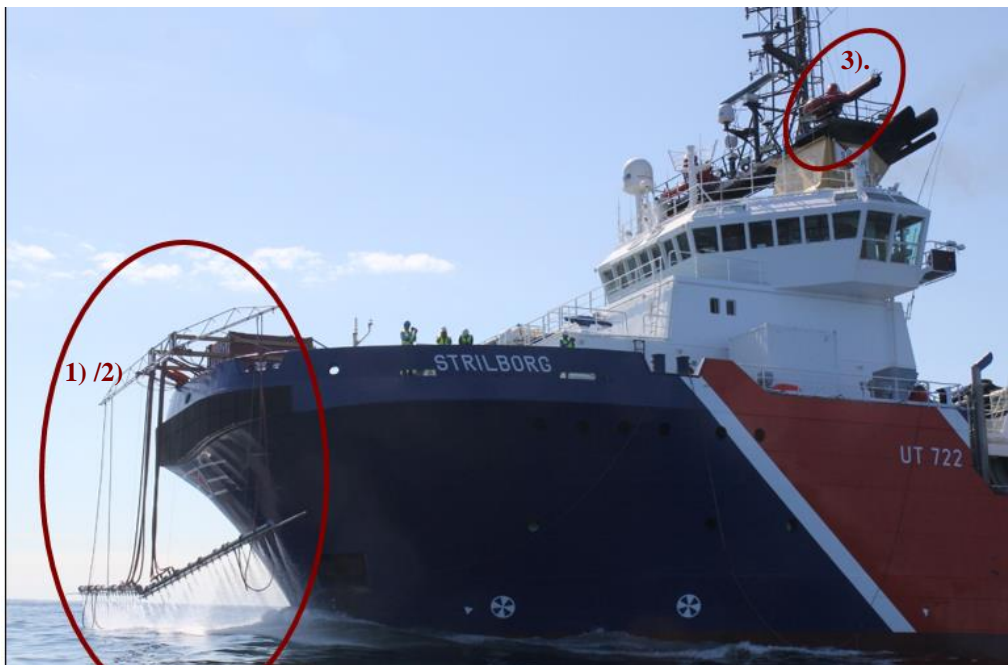
Figure 7-5 Response systems installed on MS Strilborg for treatment of thin oil films: 1): High/low dosage dispersant spraying system, 2): High capacity water flushing boom, 3): Fi-Fi monitors
