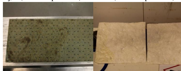
Figure 6-6 Adhesion of oil residue to sorbent pads at the end of the experimental period
