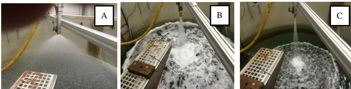
Figure 7-2 Testing of nozzle concepts in the SINTEF tower basin A) full jet 120°, B) Flat jet (25°)-most promising C) Full cone nozzle (less penetration-no further testing)
