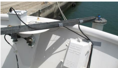
Figure 3 Bow mounted down-looking wave radar with vertical accelerometer for motion compensation.
