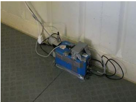
Figure 2 Fiber optic gyro with rate gyro and heave accelerometer.
