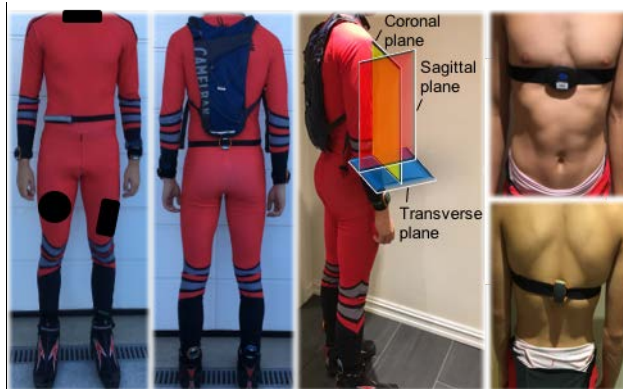
Fig. 1 Location of the seven triaxial IsenseU-ski sensors and sensor orientation relative to the skier
