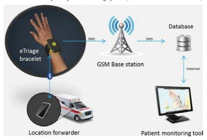
A single button is used for all operations. If the bracelet is off, a long press on the button will switch it on. If it is already on, a long press will unlock the current triage level, allowing the user to select a new triage level using short presses on the button. To avoid leaks, and make the bracelet more robust and easier to handle, charging is inductive and no wires are needed.
