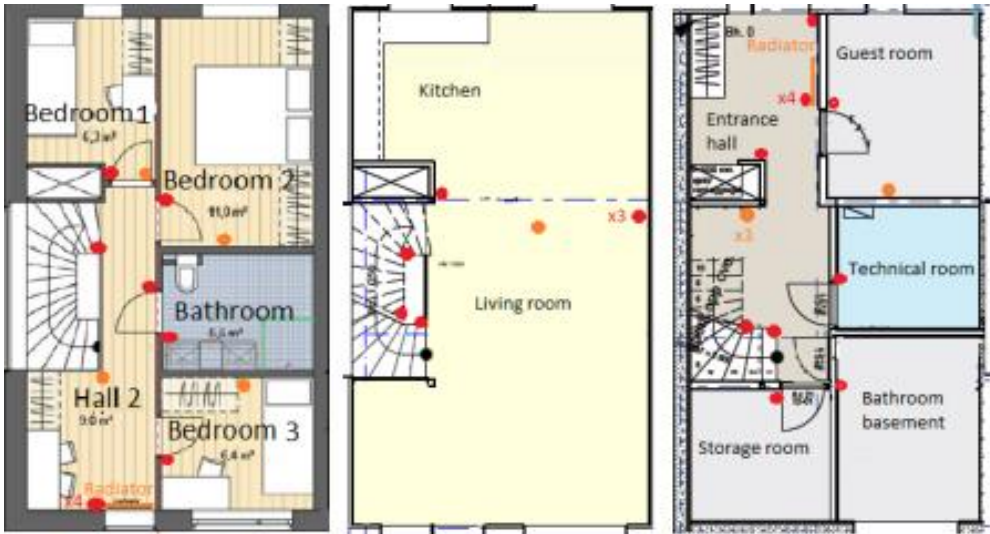
Figure 3.4 Picture (image Interiørfoto AS) and layout of House 2: first floor (left), ground floor (centre) and basement (right) with north pointing upwards [24]; orange points show the positioning of air temperature sensors in the ventilation terminal devices and the red inside the rooms.
