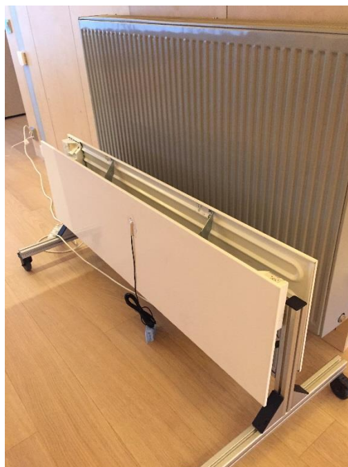
Figure 7.3 Twin electric radiators and the original waterborne radiator.
