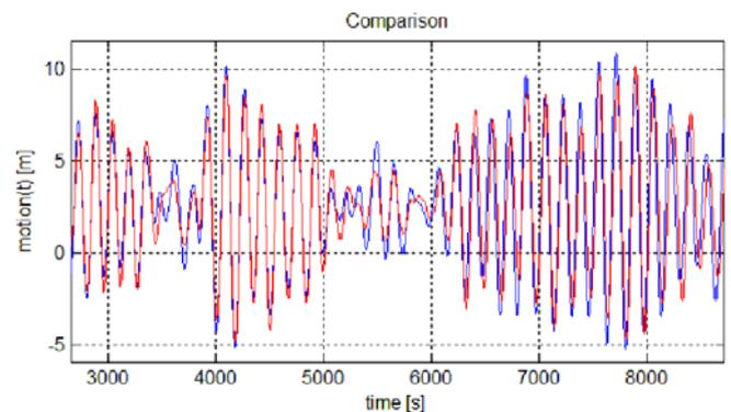
Figure 1: Comparison betw. measured slow drift surge motion (blue line) and reconstructed from the identified empirical QTF (red line).
