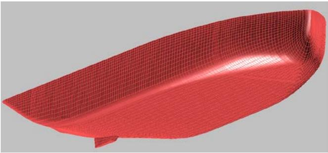
Figure 3: FPSO hull mesh for MULDIF hydrodynamic calculations.
