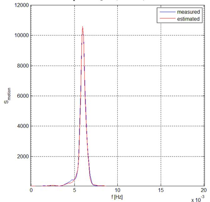
Figure 2: Spectra of low frequency surge motion. Comparison between exp. spectra (blue) and reconstructed spectra calculated from the identified QTF (red).
