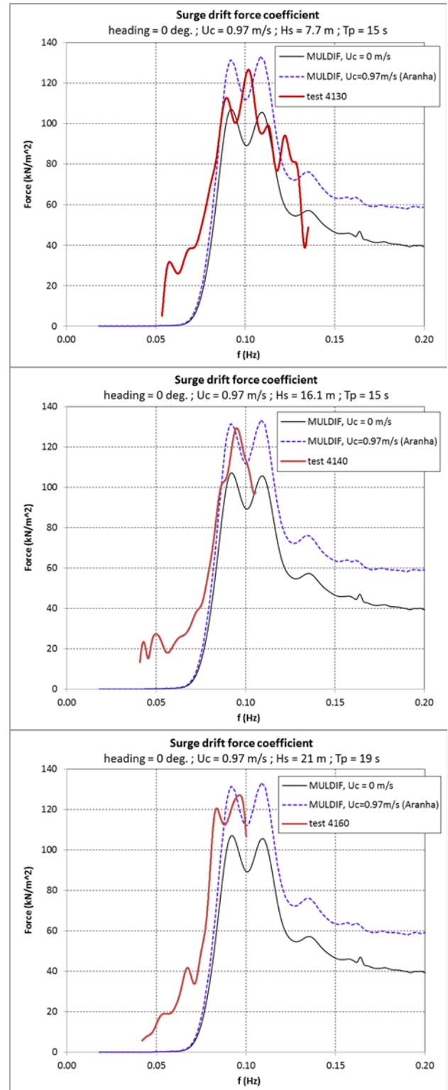
Figure 5: Surge wave drift force coefficients for three seastates with increasing  $H_s$  and  $U_c = 0.97$  m/s. MULDF results for  $\Delta f = 0$  and empirical coeffs. for  $\Delta f = 0.0051$  Hz.
