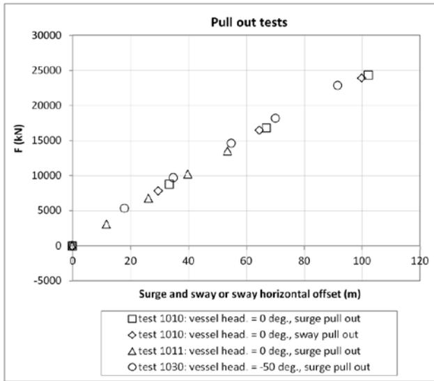
Figure 9: Exwave FPSO mooring system horizontal restoring force from pull out tests
