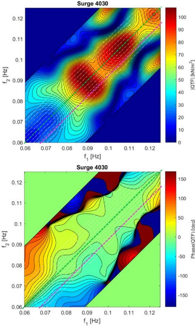
Figure 8: Surge force full QTF estimate contour plot example. Hs=7.7m, Tp=15s, head. = 0 deg., Uc=0. Upper graph: modulus; Lower graph: phase.
