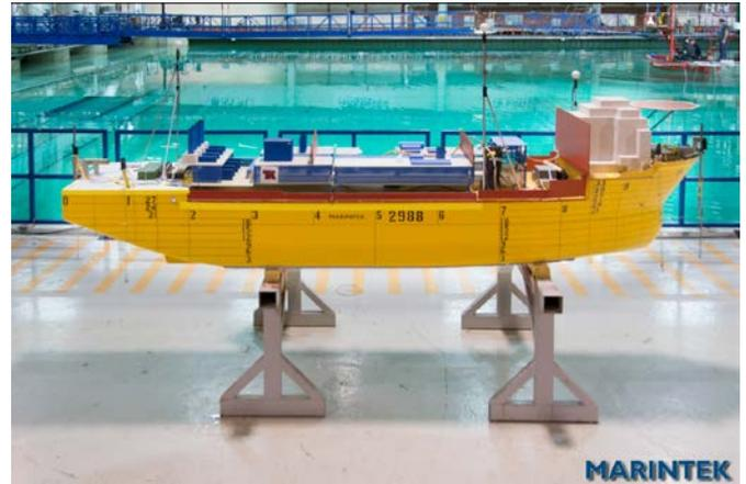
Figure 1: EXWAVE FPSO 1:70 scaled model.
