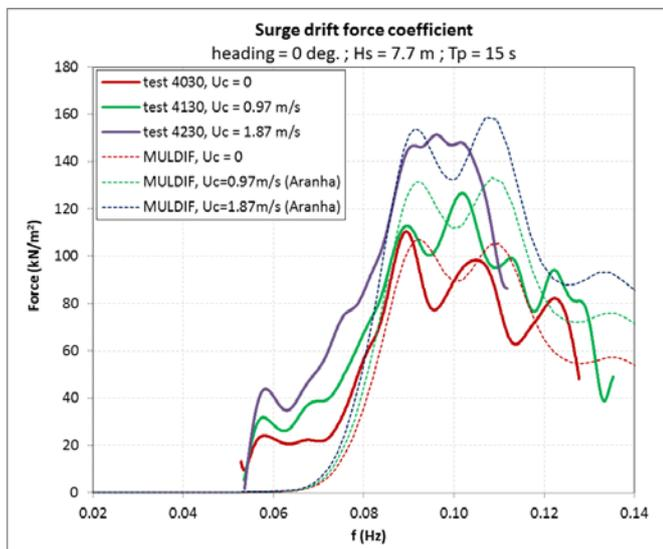
Figure 6: Comparison of surge wave drift force coeffs. for one moderate seastates and three current velocities. MULDF results for  $\Delta f = 0$  and empirical coeffs. for  $\Delta f = 0.0051$  Hz.
