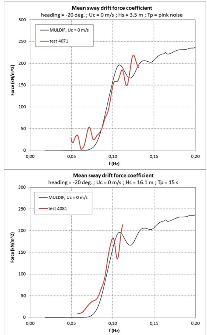
Figure 7: Comparison of sway wave drift coefficients for two seastates. Vessel head. = -20 deg.,  $U_c = 0$ . MULDF results for  $\Delta f = 0$  and empirical coeffs. for  $\Delta f = 0.0038$  Hz.
