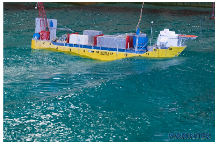
Figure 4 FPSO model (scale 1:60).
