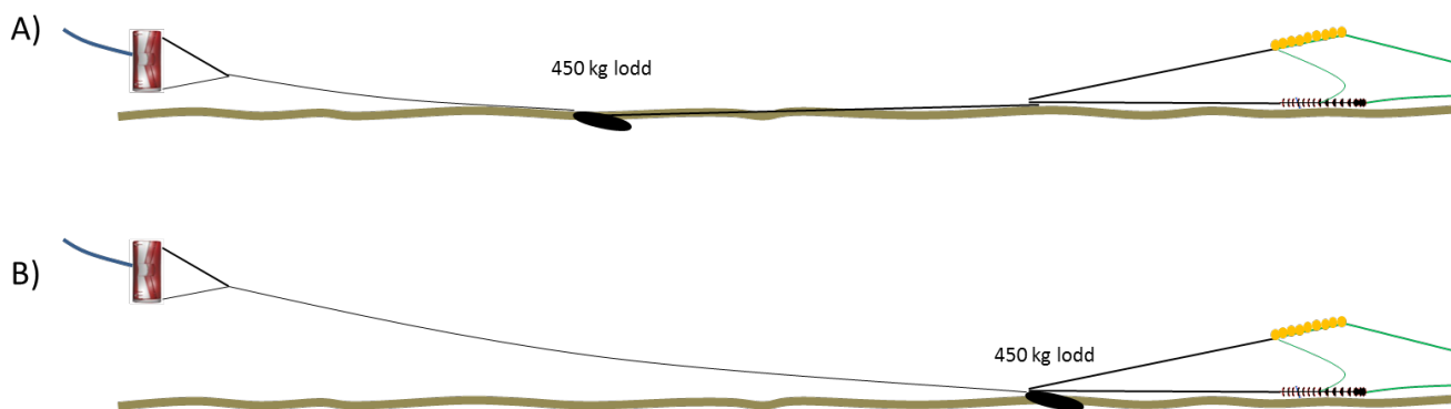
Figure 8. Sketch of the rigging of the trawl: A) The 450 kg weight is fixed behind the doors (45 m in front of the ground gear), and B) The weight is fixed in the joint between the sweep and the ground gear.
