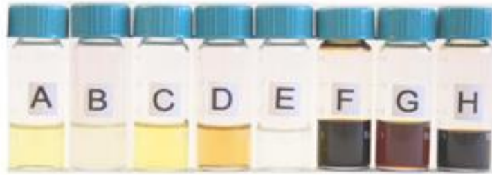
Figure 3-1 Visual presentation of the project oils. Condensates (A–E) were clear/yellow, light oils (F–G) were dark red/brown. A: Skarv, B: Atla C: Alve, D: Marulk E: Ormen Lange F: GjØa G: Vale H: Statfjord C
