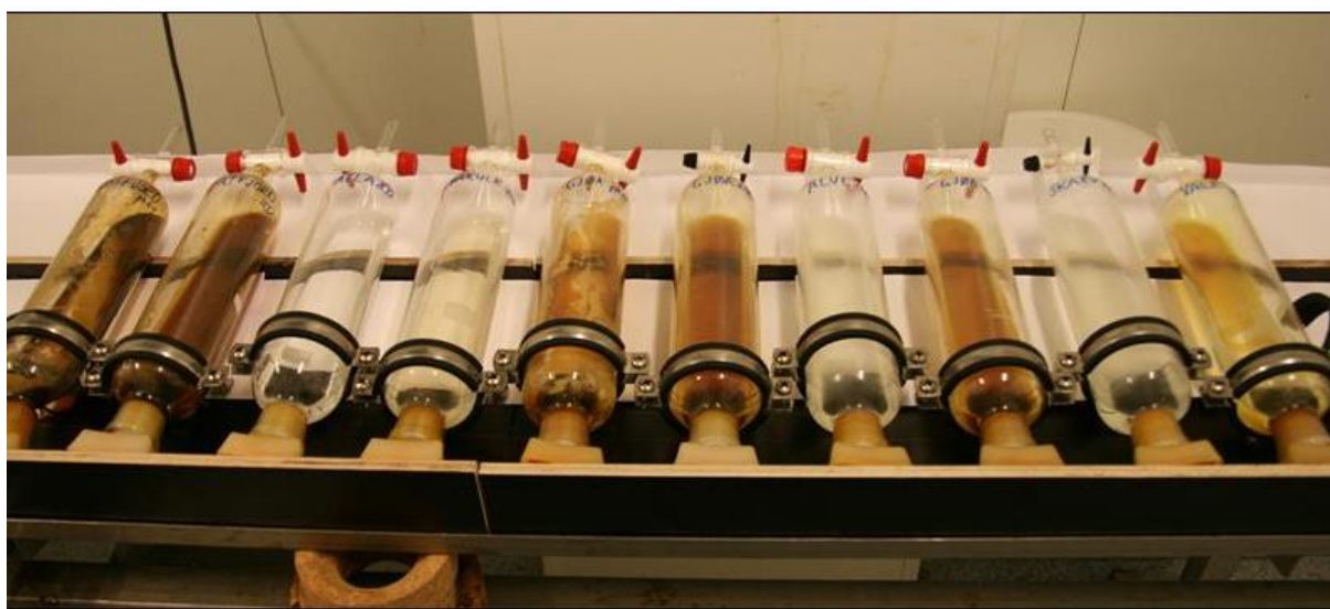
Example from the "Tilting cylinder method" of different oils/residues with use of tilting energy.
